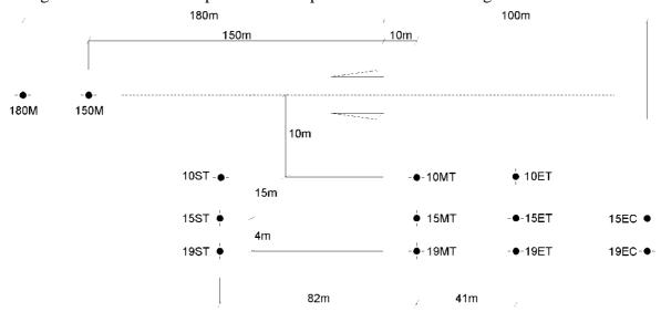
The ramp must be parallel to the jump course and slightly open. The tolerance for standard jumping is between  $+1.00^{\circ}$  and  $+2.50^{\circ}$  open. The tolerance for ski flying is between +5.00 and +7.00 open. Open means that the low end of the ramp is turned toward the jump course. The basis of the jump course is the 15ST-15MT line.
